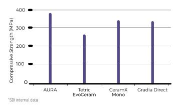
The unique morphology of the UHD filler provides an extremely high strength interface that can withstand high compressive forces.
