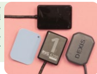
Figure 1: Large sensors (top) can be difficult to position. Options include phosphor plates and smaller sensors.
