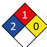
Note: The hazard category numbers found in GHS classification in section 2 of this SDSs are NOT to be used to fill in the NFPA 704 diamond. Blue = Health Red = Fire Yellow = Reactivity White = Special (Oxidizer or water reactive substances)
